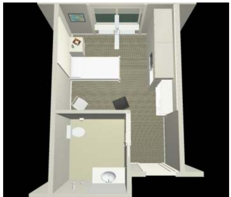
Above: Aged care rooms can be easily rearranged to either provide extra living space and facilities for an ambulant resident, or a space optimized for care of frail aged residents. In the latter case, the room can be optimized to minimize Occupational Health and Safety hazards for the carer.
